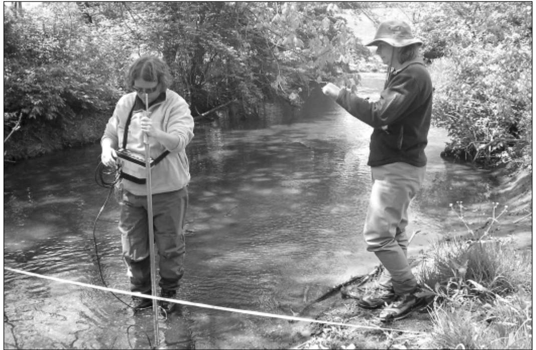
Jessica Schuster (left) and Andrea Fredenburg, of the Division of Water, measure and record stream velocity on Elkhorn Creek in Fayette County. Stream velocity is the speed at which the water is passing a certain point per unit time. Division of Water photo
